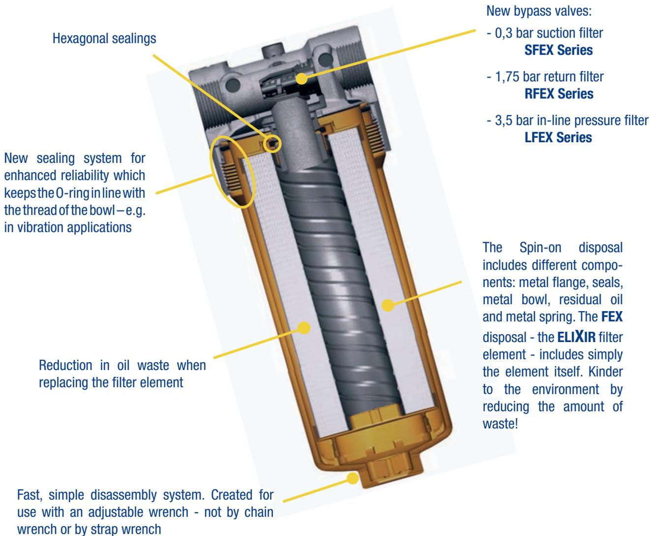
The Spin-on disposal includes different components: metal flange, seals, metal bowl, residual oil and metal spring. The **FEX** disposal - the **ELIXIR** filter element - includes simply the element itself. Kinder to the environment by reducing the amount of waste!
