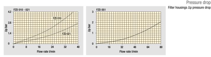
The curves are plotted using mineral oil with density of 0.86 kg/dm<sup>3</sup> in compliance with ISO 3968. ∆p varies proportionally with density.
