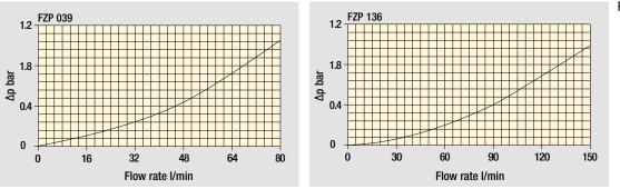
The curves are plotted using mineral oil with density of 0.86 kg/dm<sup>3</sup> in compliance with ISO 3968. ∆p varies proportionally with density.
