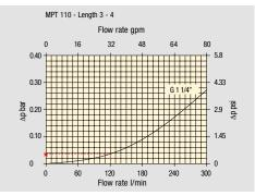
Filter housings ∆p pressure drop. The curves are plotted using mineral oil with density of 0.86 kg/dm<sup>3</sup> in compliance with ISO 3968. ∆p varies proportionally with density.
