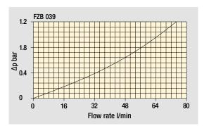
The curves are plotted using mineral oil with density of 0.86 kg/dm<sup>3</sup> in compliance with ISO 3968. Δp varies proportionally with density.
