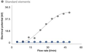
Under standard working conditions, the potential goes from tens of kV to zero, clearly showing the effectiveness of our dissipative filters.
