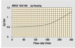
Bypass valve pressure drop
