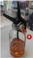
Connect the LPA3 waste outlet quick-release attachment (C) and then connect the waste hose to a waste receptacle (B)
