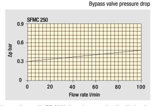
The curves are plotted using mineral oil with density of 0.86 kg/dm³ in compliance with ISO 3968.  $\Delta p$  varies proportionally with density.
