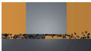
CONTAMINATION IN PRESENCE OF NARROW TOLERANCES
