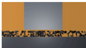
CONTAMINATION IN PRESENCE OF LARGE TOLERANCES
