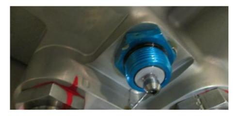
Check integrity of this seal. If it appears damaged in any way, this should be replaced prior to fitting the adaptor.
