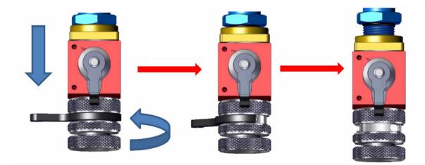
WARNING: During disengagement, DO NOT allow the adapter to pass any distance from the vertical. It is imperative that the adaptor is kept fully vertical.
