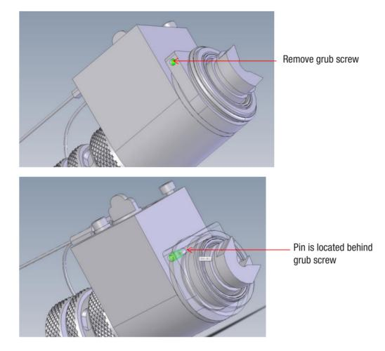
8.2.3 Remove the collar from the adapter. Store this and the pin in a safe place
