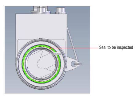
**8.2.1** Carefully remove the collar to allow access to the seal
