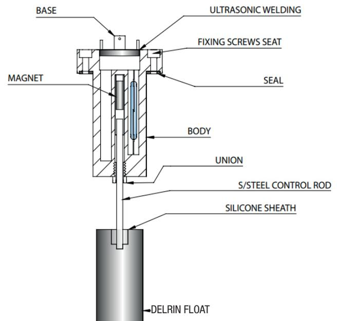
On request the float can be supplied with through hole and therefore be positioned in the required position without having to cut the rod (which can therefore be as long as the height of the tank).
