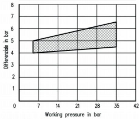
DIFFERENTIAL PRESSURE OF IPH-150 PRESSURE SWITCH
