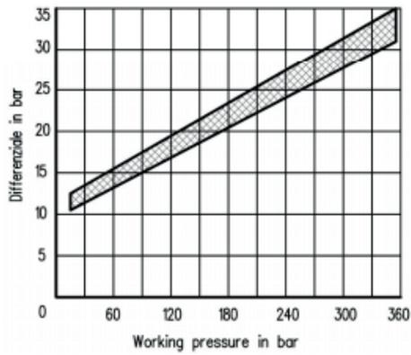
DIFFERENTIAL PRESSURE OF IPH-630 PRESSURE SWITCH
