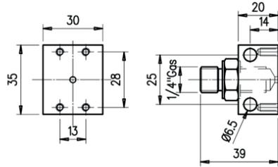
It allows the pressure switch mounting:
