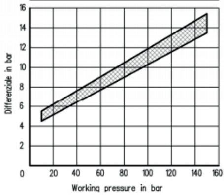
DIFFERENTIAL PRESSURE OF IPH-250 PRESSURE SWITCH
