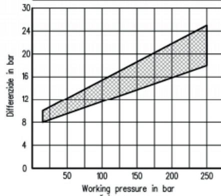
DIFFERENTIAL PRESSURE OF IPH-350 PRESSURE SWITCH
