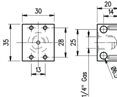
It allows the pressure switch mounting: panel-mounted adaptor by using n.2  $\varnothing 6.5$  holes.
