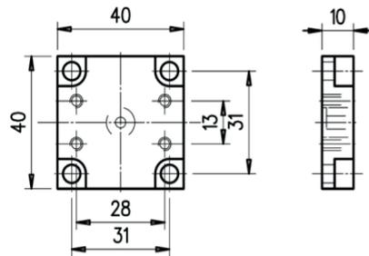
It allows the pressure switch mounting:
