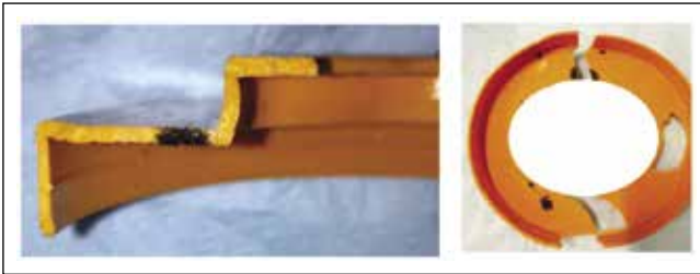
> FIG. 8 - Detail of the bead core of a glass filter damaged by drains
