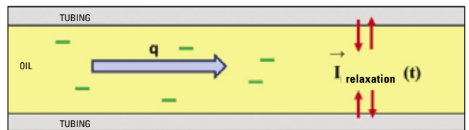
> FIG. 5 - Charge relaxation in the pipes
